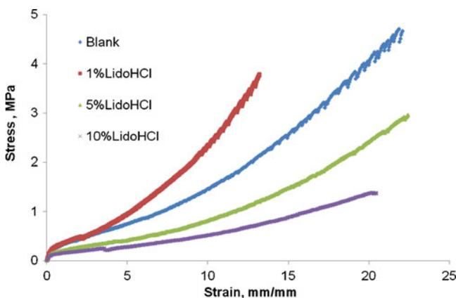
**Fig. 3** Stress–strain curves of silicone bands with different drug loadings (From top: 1%, blank, 5% and 10%)
