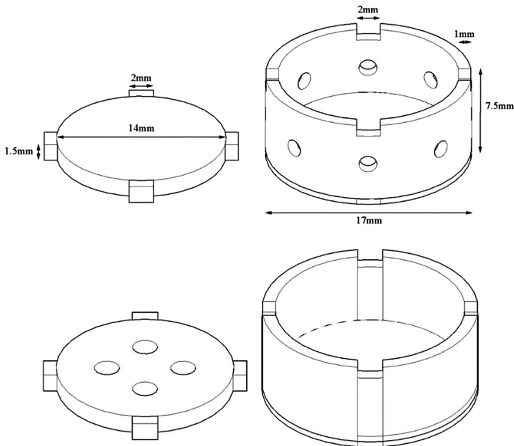
**Figure 1.** 3D model of rhodamine B containing tablets. Top: lid and tablet body with holes at the side. Bottom: lid with holes and tablet body. Both tablets have the same dimensions.
