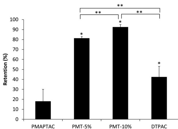
**Fig. 4** Retention of characteristic peaks of antimicrobial coatings after the abrasion test. Data represents the standard deviation of three tested samples.  $p$ -value < 0.05 indicates statistically significant, and \* shows significance between the QAS coated samples and PMAPTAC coated samples, while \*\* shows significance between different QAS coated samples.
