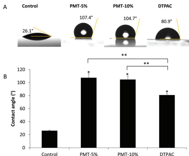
**Fig. 3** (A) Water droplets on the surfaces of uncoated and coated glass. (B) Contact angles of the surfaces of uncoated and coated glass. Data represents the standard deviation of at least three tested samples.  $p$ -value < 0.05 indicates statistically significant, and \* shows significance between coated samples and control, while \*\* shows significance between different coated samples.
