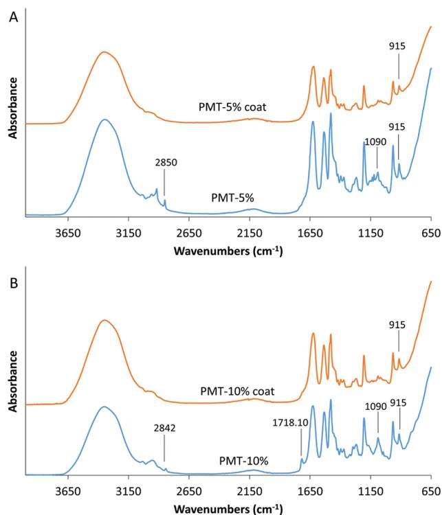
Fig. 2 ATR-FTIR spectra of: (A) PMT-5% copolymer and coating; (B) PMT-10% copolymer and coating.
