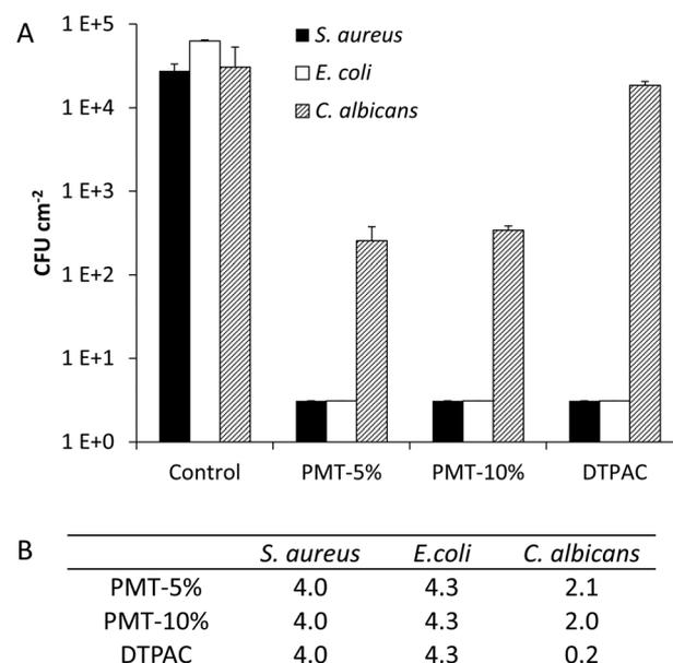
**Fig. 7** Variable bacterial counts of QAS coatings against *S. aureus*, *E. coli* and *C. albicans* after 24 hours of exposure to coated glass cover slips (A) and the corresponding numerical values (B).
