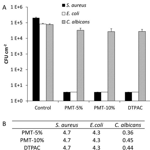
**Fig. 8** Variable bacterial counts of QAS coatings against *S. aureus*, *E. coli* and *C. albicans* after 24 hours of exposure to coated Lava restoratives (A) and the corresponding numerical values (B).
