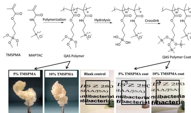
**Fig. 1** Synthesis scheme of QAS copolymers and coatings. The physical appearances of synthesized QAS copolymers of PMT-5% (5% TMSPMA) and PMT-10% (10% TMSPMA) are shown, with the optical transparency of QAS copolymer coatings in comparison to the control.
