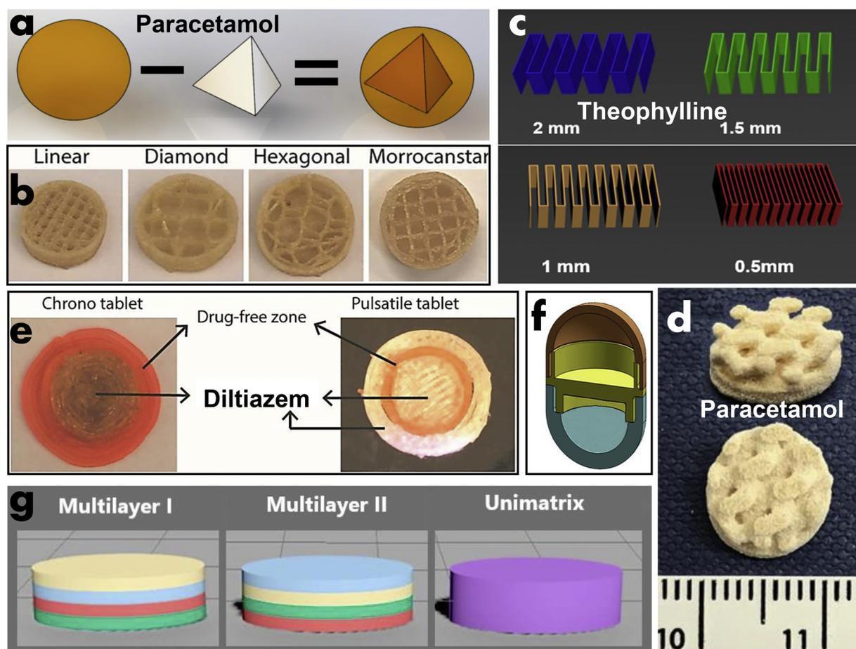
**Fig. 1.** Oral dosage forms created by AM. (a) Model of 3D printed shell with convex drug release profile. (b) Various infill patterns created by 3D printing. (c) Computer-aided design file of novel radiator-like design. (d) 3D printed bilayer tablet consisting of multiple release profiles. (e) 3D printed “chrono tablet” and “pulsatile tablet”. (f) Capsule consisting of two separate compartments. (g) Computer-aided design file of different architectures for a polypill.
