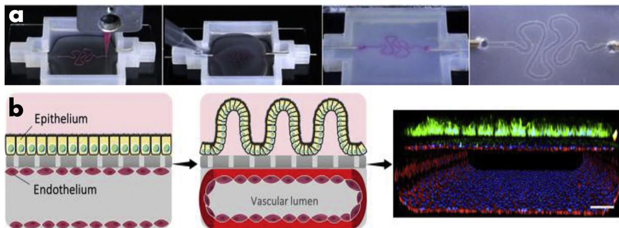
**Fig. 6.** 3D printing of cellular models. (a) Renal microfluidic device created using 3D printed sacrificial Pluronic® ink. (b) Schematic of intestinal epithelium and endothelium differentiating to form a villus epithelium and vascular lumen respectively, and an immunofluorescence micrograph visualising this.
